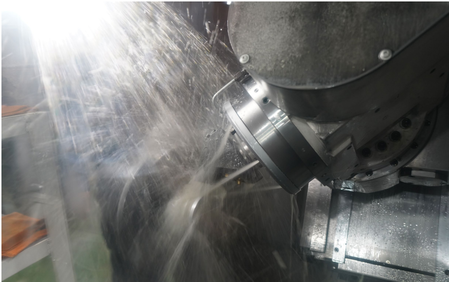
Above: lens polishing. Below: CNC machining of mechanical components.
