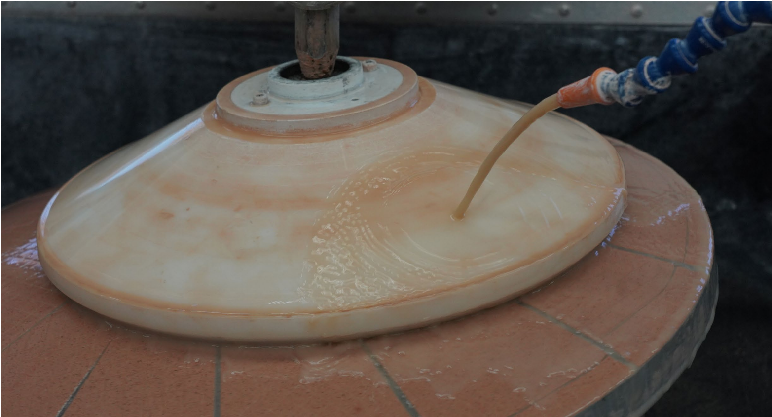
Above: lens polishing. Below: CNC machining of mechanical components.
