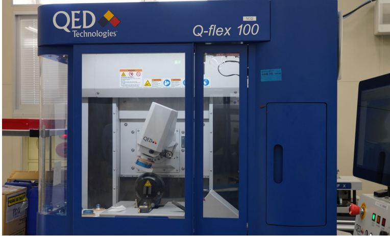
Q-flex 100 MRF (Magnetorheological Finishing) freeform polishing machine can work on elements up to approximately 125 mm diameter
