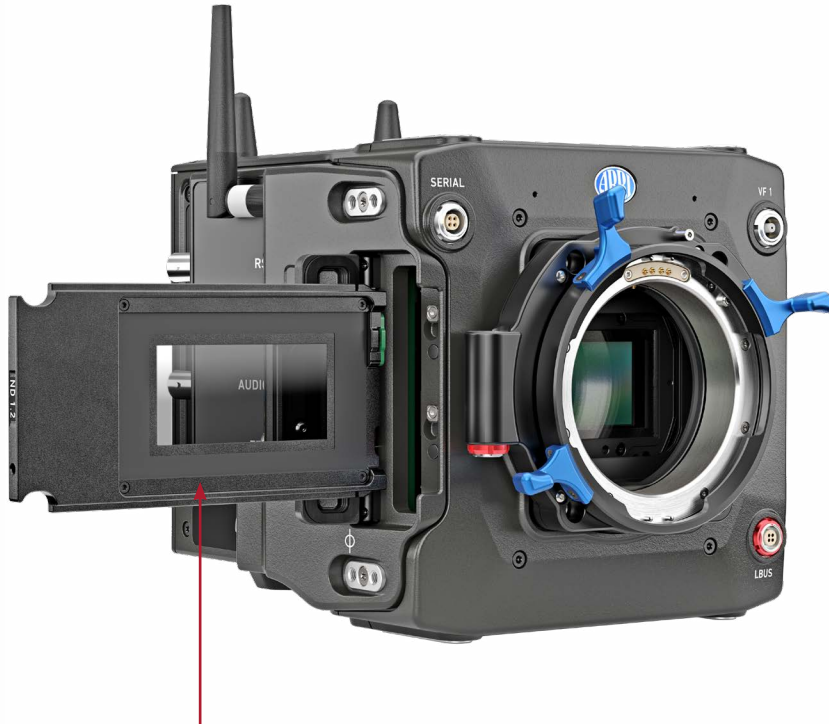
Filter Cartridge removed
