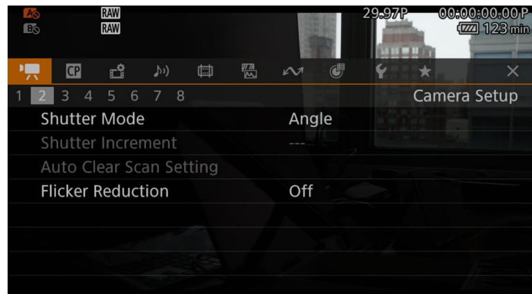
2. Set Shutter Mode to Angle, as in 180° shutter and not 1/48th second.
