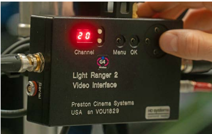
The Light Ranger 2 Video Interface connects to your monitor and provides a video overlay showing zones of focus. Photos by HD-Systems.
