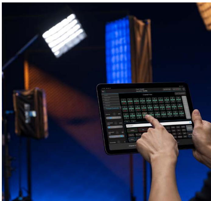
Nanlink app on tablet controlling Nanlite PavoSlim fixtures
