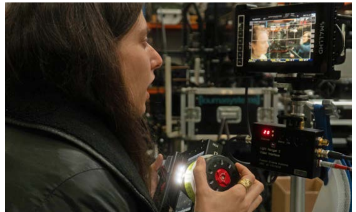
The Light Ranger 2 Video Interface connects to your monitor and provides a video overlay showing zones of focus. Photos by HD-Systems.
