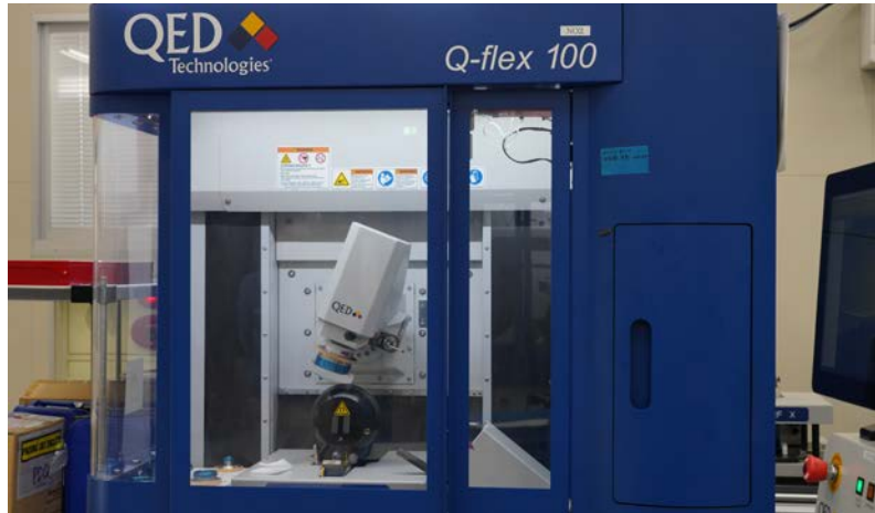
Q-flex 100 MRF (Magnetorheological Finishing) freeform polishing machine can work on elements up to approximately 125 mm diameter
