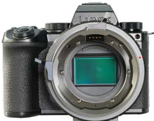
S5IIX with Leitz L to LPL Adapter and LPL to PL Adapter. You can tell the difference because the LPL to PL Adapter has winged tabs.
