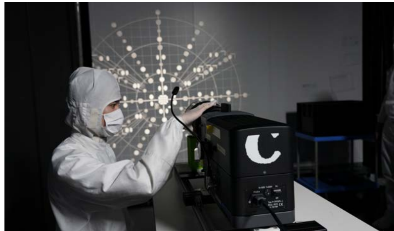
Checking lenses on a Chrosziel TP-7 projector
