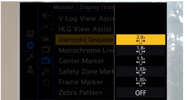
The S5IIX has one of the more advanced Anamorphic Desqueeze capabilities of any Full Frame hybrid mirrorless camera: 1.3, 1.33, 1.5, 1.8, 2.0x.
