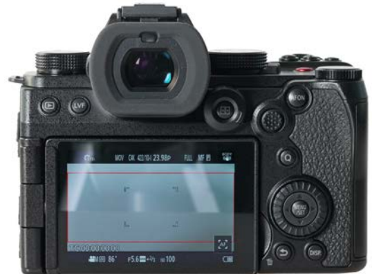
Rear view. Monitor data shows that we're recording Cinema 4K .MOV, Full Sensor Area, at 23.98 fps, with Manual Focus, Program Exposure of F5.6 at 86 shutter angle, ISO 100 and 2.339:1 aspect ratio.
