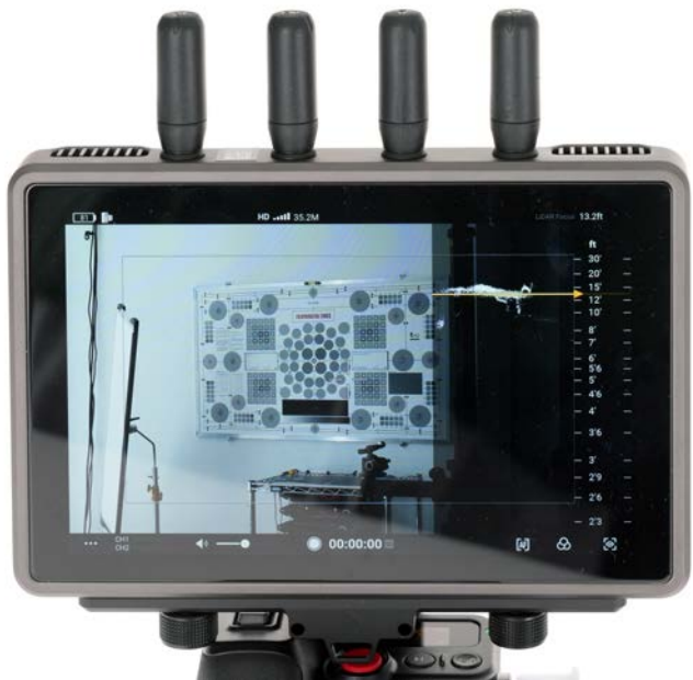
11. Success. You have saved the lens profile. The screen should look like this. The yellow arrow points to the focus distance you have set with your Hand Unit. The white blob to the left of the arrow is the recommended distance of the LiDAR rangefinder.
