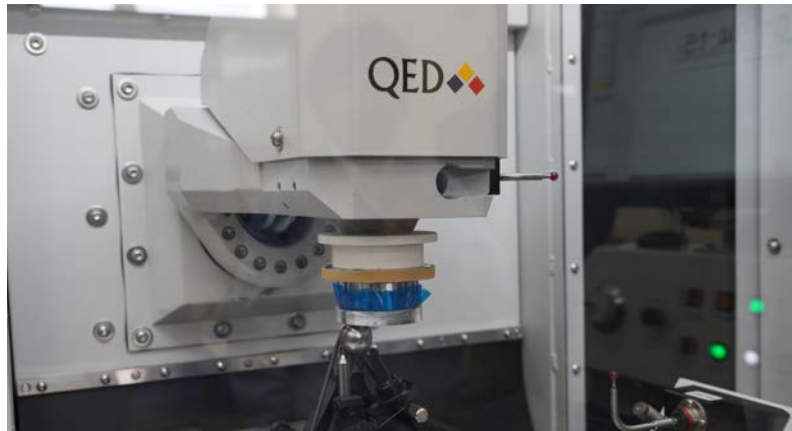
Q-flex 100 MRF (Magnetorheological Finishing) freeform polishing machine can work on elements up to approximately 125 mm diameter
