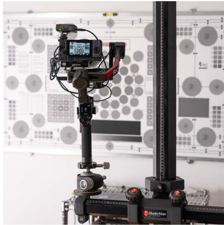
10. If you're not setting up in a rental house prep bay, you will save a lot of time and aggravation by attaching the focus chart or target to a wall and moving the Ronin RS4 Pro setup on a tripod, dolly or rolling pedestal.
