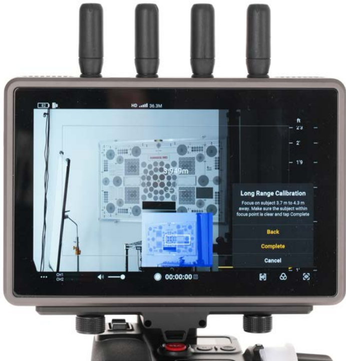
9. The next step is Long Range Calibration. Back away from your focus chart until it is 3.7 to 4.3 m (12.1 to 14.1 ft) away. Focus the Hand Unit until the image is sharp, and touch CONFIRM.
