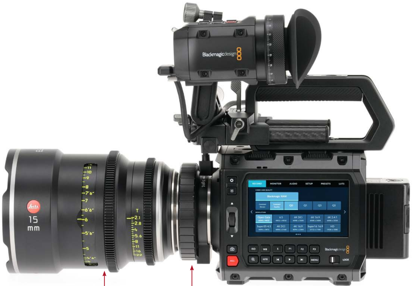
Leitz ELSIE 15mm T2.1 Full Frame Prime Lens, LPL Mount
