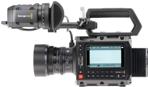
EVF mounted forward for shoulder-resting handheld setups.
