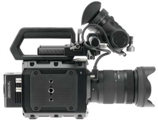
This is the standard right side plate. To remove, undo 4x 2.5mm hex screws.
