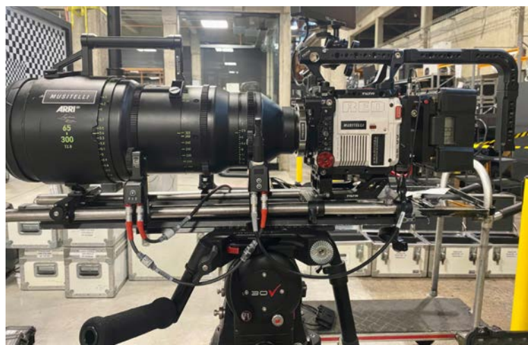
Signature Zoom (LPL) on RED Raptor with TILTA RF to LPL adapter.
