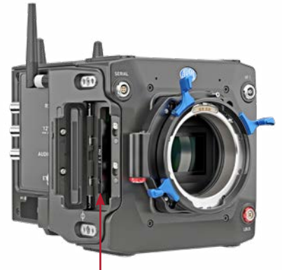
Filter Cartridge inside: here's an ND1.2.
